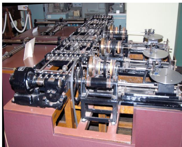
Fig. 2: Differential Analyzer used at Osaka University and is now preserved by Tokyo University of Science
