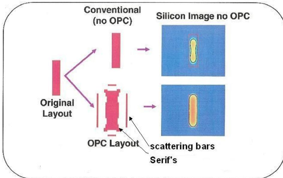
In the above illustration, the desired chip image is just a vertical rectangle (Original Layout). However, if you provide that on the mask (no OPC) you get a fuzzy oval, lacking the squared corners of the original. On the other hand, you can add OPC (OPC Layout) to the mask such as scattering bars and serifs. This results in chip features looking much more like the original layout even though it is not close to what is on the mask itself.
