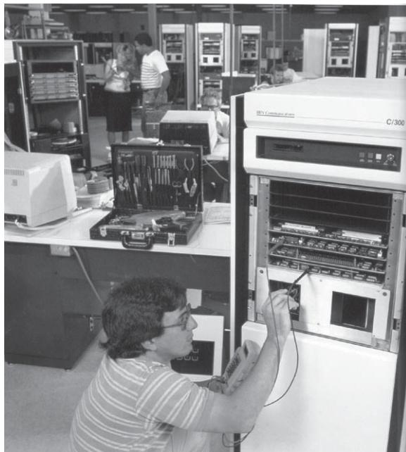
Figure 6.8 A BBN Communications C/300 packet switch being checked before shipment.
