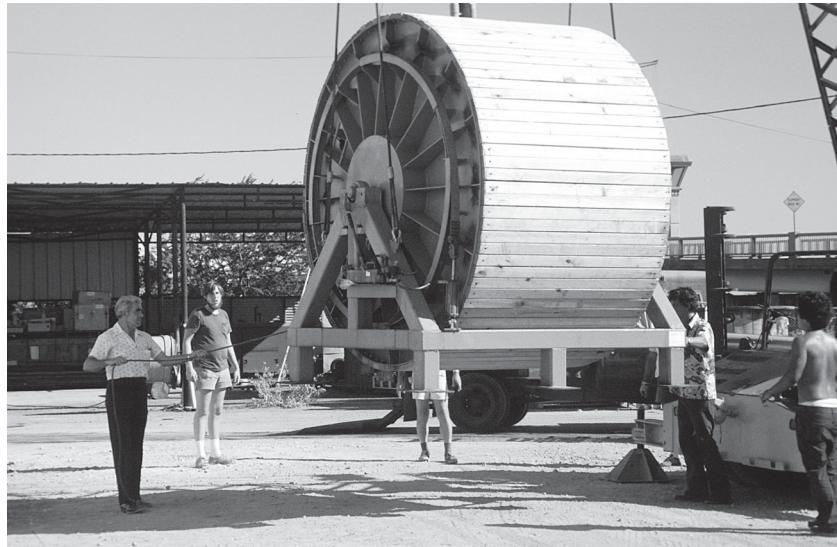
**Figure 10.12. Submarine towed-line array installed in its winch is lifted aboard the RV Washington. (Photo courtesy of Joe Walters Jr.)**
