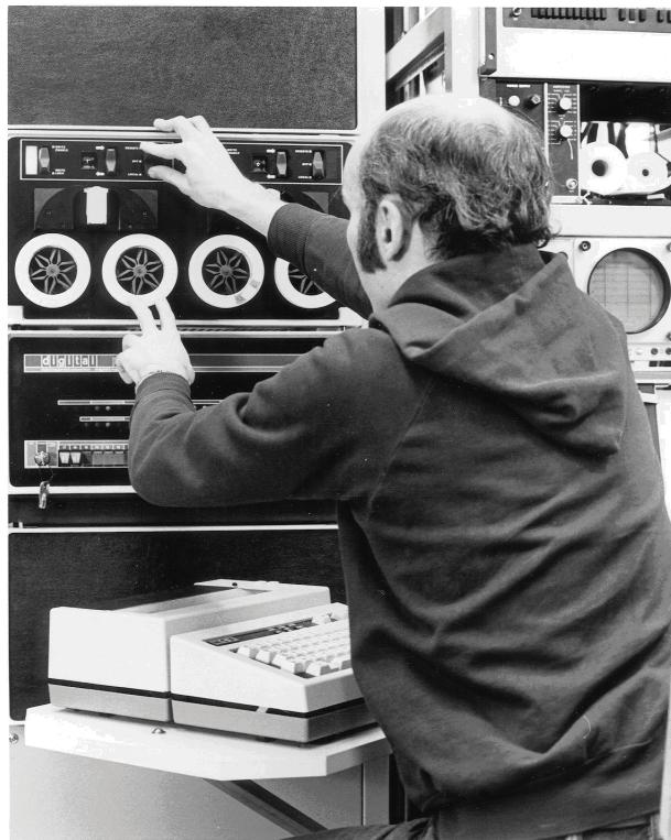
**Figure 10.5. Bob Pyle loading magnetic DECTape for the PDP-11/20. (Photo courtesy of Douglas Steele.)**
