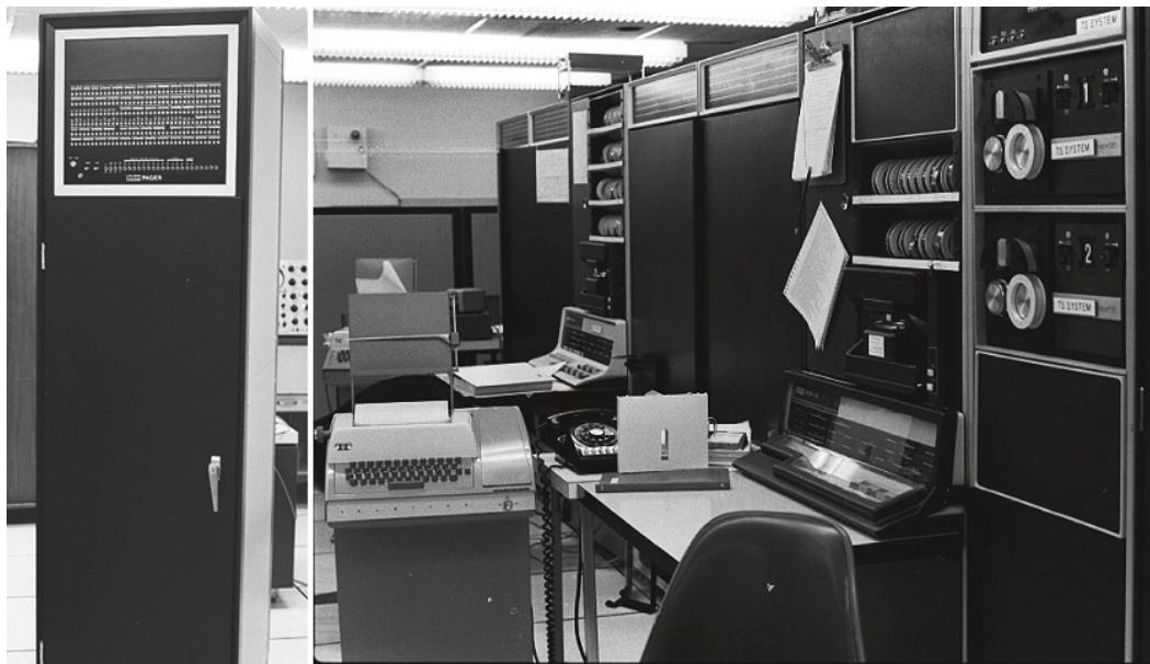
**Figure 21.1.** TENEX pager and DEC-KA10 machines used for TENEX development and time sharing, circa 1970. (Photos courtesy of Dan Murphy.)
