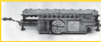
1674 Gottfried Leibniz builds the "Stepped Reckoner," a calculator using a stepped cylindrical gear.
